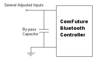
The above circuit model illustrates the By-pass capacitor that we will use as a primitive noise filter.
