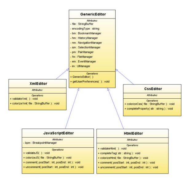
• Main controller class of the editors which is created once on the start of the program. It handles opening new tabs, closing existing ones and switching between them:
