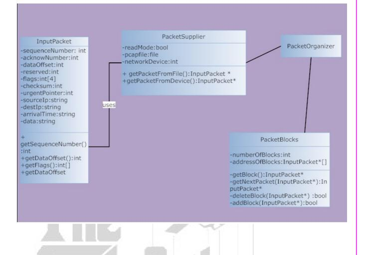
*InputPacket* class is a generic packet class. It contains a lot of TCP values. These values are used for filtering and ordering.
