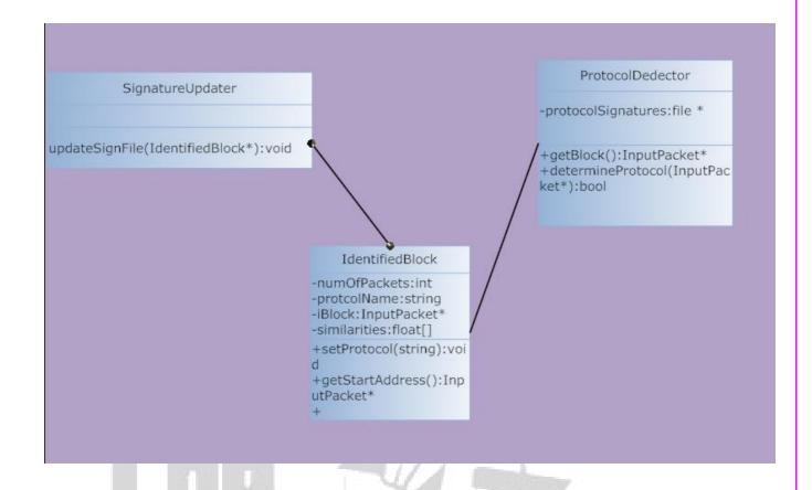
**ProtocolDedector** class gets a packet block(group of related packets) from **PacketBlocks** class. This is the most important class of the project, because using pattern recognition techniques, the protocol of packets are determined here. Also we keep the signature of protocols in a file. After protocol was identified this class produces an output: **IdentifiedBlock**
