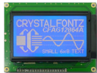
Figure: Above LCD has 128x64 resolution.
