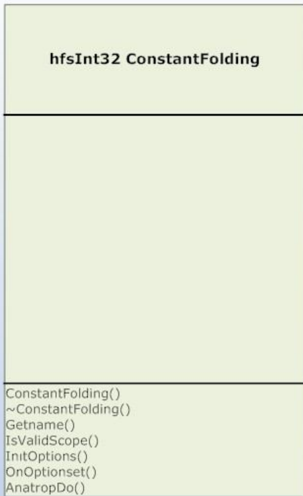
Diagram 1.c ) class diagram for constant folding optimization
