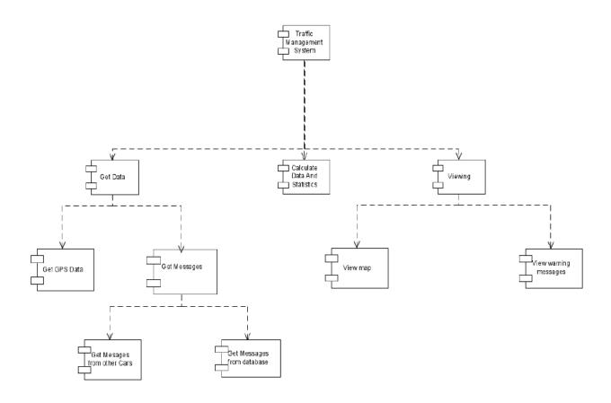
Generally, it can be said that Get Data, Calculate Data And Statistics and Viewing modules are going to be tested separately and then their integration testing will also be done.
