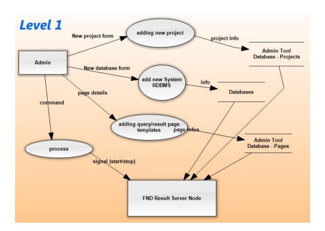
Level 1 Data Flow Diagram represents the flow of data while the admin uses the administration tool. This Data Flow Diagram consists of 4 parts.
