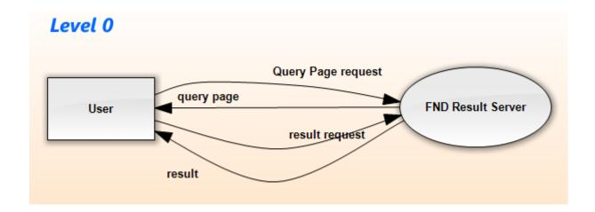
Level 0 Data Flow Diagram represents the flow of data in the process of usage of the system by an end user. In this Data flow diagram actually there are two parts. First one is to show the user the query page, the second one is the result page.
