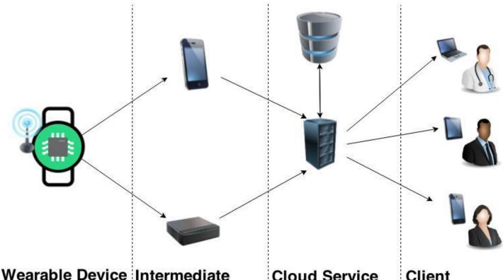
A wearable device is an equipment Devices placed on patient's wrist. Health data is measured via physiological sensing and sent to the paired device using bluetooth®.
