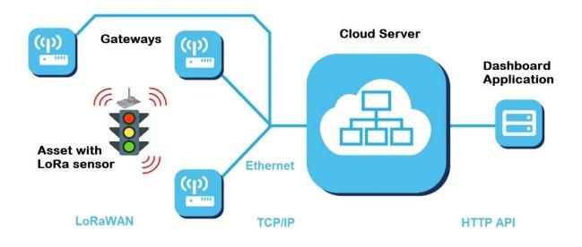
LoRa sensors transmit data to gateways via wireless communication LoRa protocol. Gateways transmit data to the cloud/remote server. By comparing the signal strength received by each Gateway, location of the assets are detected. A dashboard application shows the locations of all inventories in the system. By using a web service, notification will be sent in case of displacement of any item.
